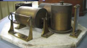
Magnetograph pieces (MCUL00386) and Octagonal box with PHOTOGRAPHIC devices of the magnetographs (MCUL00354)
